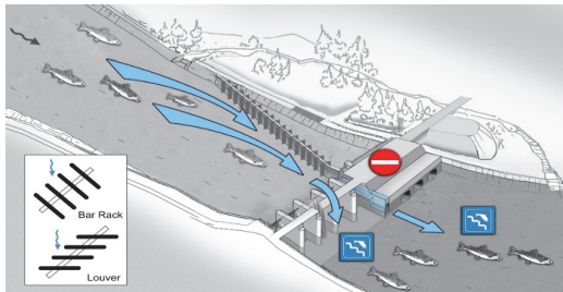
Fig. 1: Fish guidance structure with bypass at a run-of-river HPP
